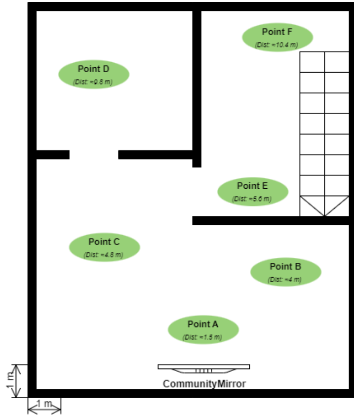
Figure 27: Floor plan of the test room with the position of the CM and the different points from where the user tries to be identified
