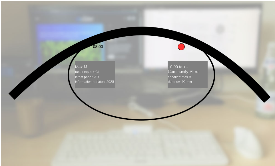
Figure 6. The overview mode of the smart glasses prototype, showing the default always-on display with suggestions for relevant sessions, persons of interest, and other contextual information. This illustration is intended to convey the visual sensation of the two screens merging due to parallax.
