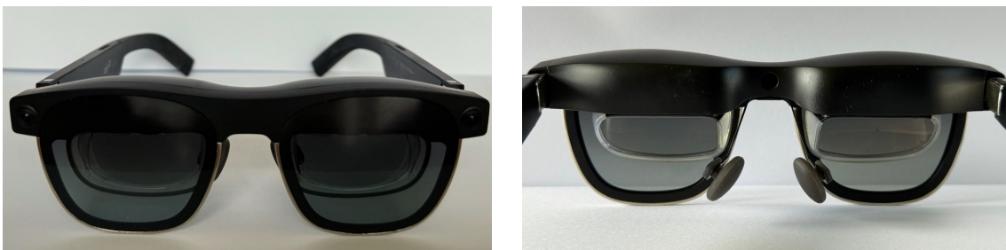
Figure 4. The smart glasses model used in this demonstration, the XREAL Air 2 Ultra, seen from the front and the back
