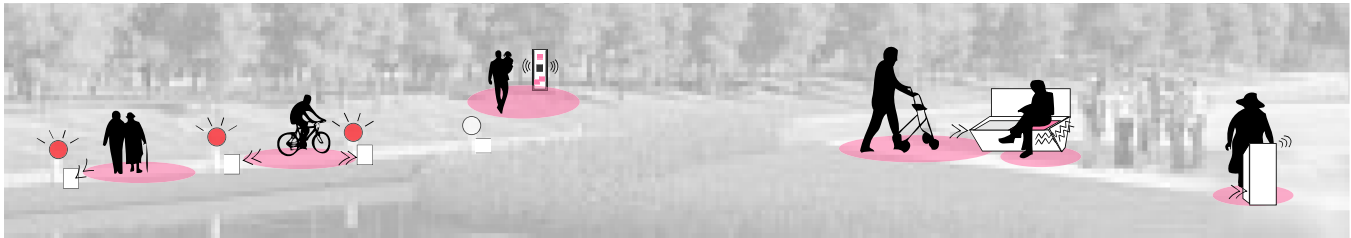
Figure 1: Information radiator network applied in urban space. From left to right: micro light signals reacting to approaching passers-by, information display, vibrating park bench signaling approaching senior, information kiosk to help overcoming barriers and to inform about the area (from [14])
